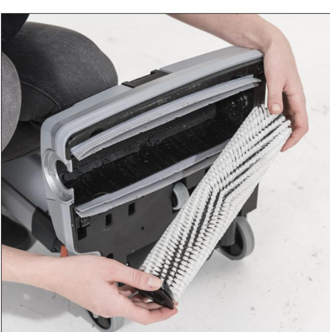
1. Check if the cylindrical brush is correctly installed and not worn out.
