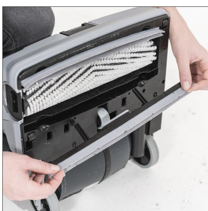
2. Check if the squeegee bars are dirty or the blades are worn or damaged.
