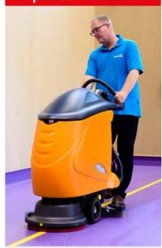
Apply the fluid while scrubbing and let the machine suck it up immediately.
